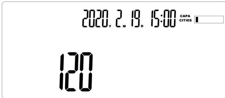
2. Press up / down / left / right buttons to set the longest recording time (1-120 minutes)
