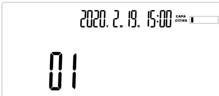
2. Press the up / down / left / right buttons to set the shortest recording time in sequence, (1-20 seconds)
