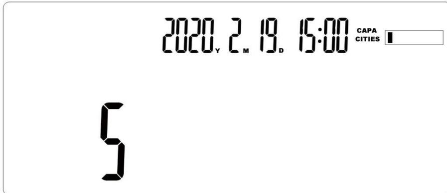
2. Press the up / down keys to adjust the brightness of the screen in order, which is divided into 5 levels (the higher the value, the higher the brightness)
