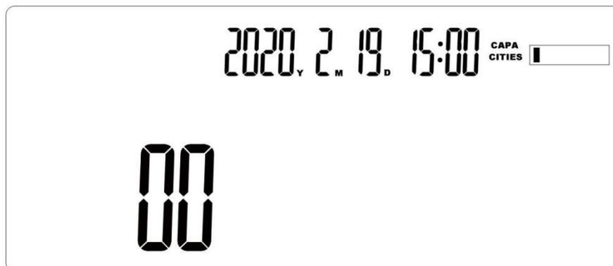
2. Press the up / down key to set the lock screen waiting time. The maximum setting time is 99 seconds.
