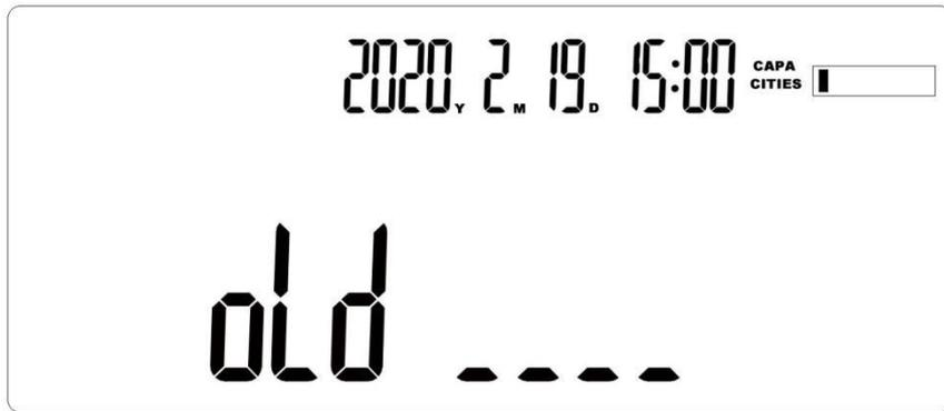
5. After the input is completed, the page of inputting new password will be displayed. At this time, it is not necessary to set, but press the confirm key twice to complete the setting. Return to the function page, and the lock screen password function will be cancelled.
