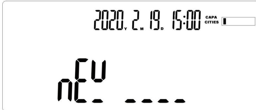
2. You can set the lock screen password from the up / down / left / right buttons according to your own needs. After setting, press the confirm key, and then repeatedly input the set password. The screen shows:
